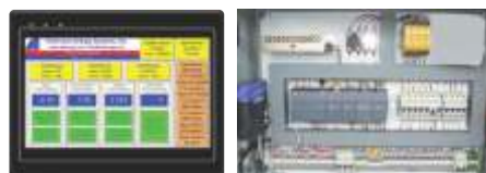
Typical Touch Screen Operator Interface. Siemens S7-1200 PLC with Ethernet Interface and DSLRouter.
